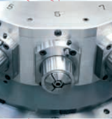
Rotary indexing table with collet chucks
