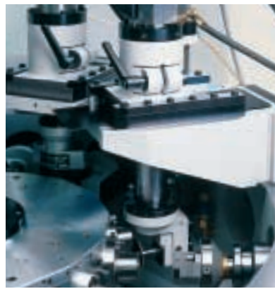
Vertical support for installing vertical machining units
